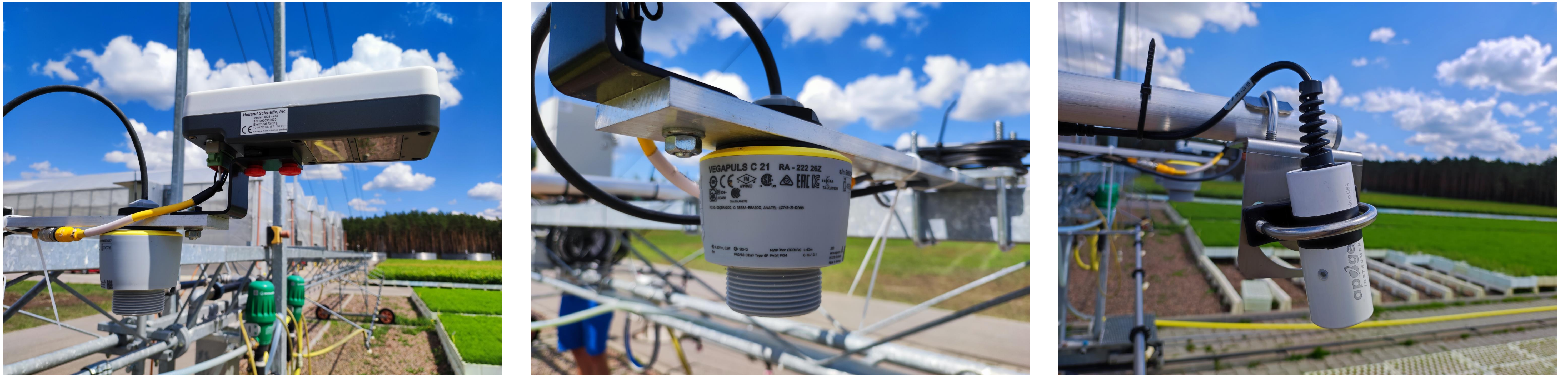
Photo 1. Plant scanners over the field of forest seedlings (from the left) ACS-435 Holland Scientific, VEGA C21 VEGAPLUS, IR SI-100SS Apogee
