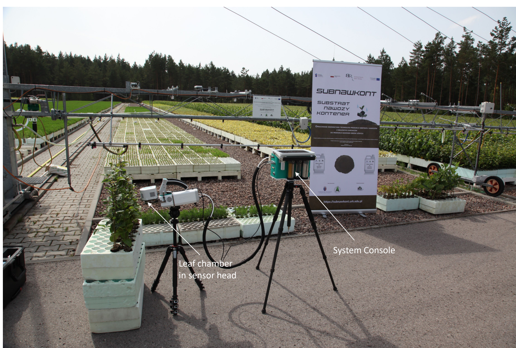
Fig. 1. Portable photosynthesis system LI-6800 during measurements in Suków Nursery Farm
